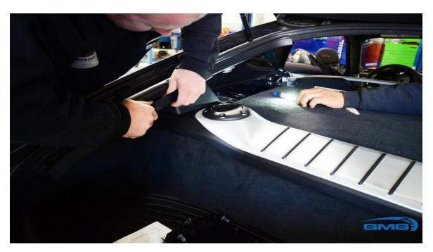
Step 4 – Remove rear trunk plastic kick panel by pulling away from the  $\frac{3}{4}$  panel toward the center inside of the vehicle.
