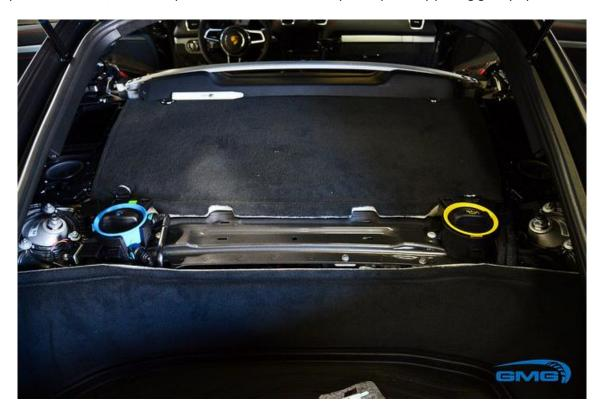
Step 6 – Loosely fit passenger side rear bar portion. Leave strut-tower nuts loose for some wiggle room. Fit driver side rear bar portion to rear strut tower and passenger side rear bar. With a little bit of antiseize tighten both rear bar sections together using the supplied 8mm hex bolts and torque to 20 ft lbs.
