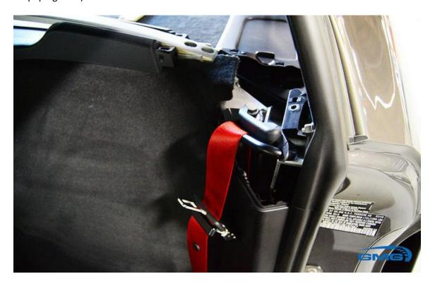
Step 3 – Remove the rear speaker plastic panels using a T-30 torx and remove panel by lifting upward/pulling toward the front of the vehicle.
