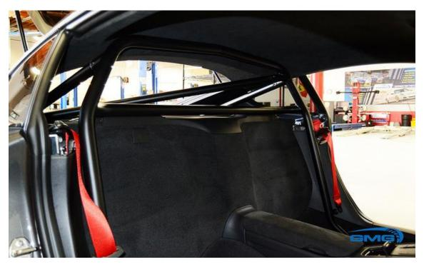
Step 8 - Once the lower seat belt portion is bolted in, the two rear upper speaker plastic panels will need to be trimmed to provide room for the harness bars attachments point on the strut towers. (REMEMBER IT'S ALWAYS EASIER TO CUT MORE, MAKE SMALLS CUTS AND TEST FIT TO ENSURE PROPER FITMENT OF PANELS)
